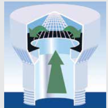
When negative pressure ceases the washer drops to seal the chamber.
