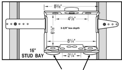
2" Right and Left Drains with knockouts
