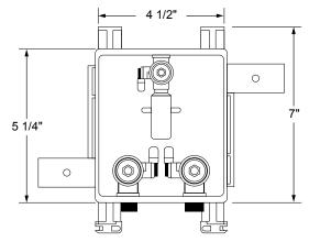
**Specifications:** Furnish and install fire-rated MultiBox Kitchen Box, combination dishwasher/ commercial ice & angle stop outlet box with extra deep faceplate for custom fit to cabinetry. Unit shall be Water-Tite product code checked below, as manufactured by IPS Corporation.
