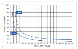
Results will vary. Performance results using a 1/3 HP (5.6A) and 1/2 HP (7.3A) pumps with 2 fully charged FloodStop 100 amp hour batteries.
